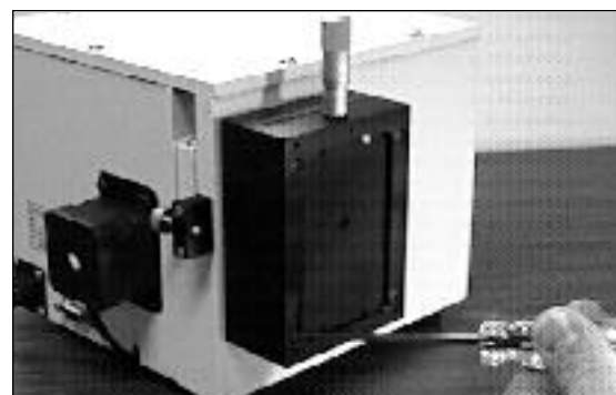
Securing the Exit Slit Assembly to the Housing Using Four (4) 8-32 Screws
